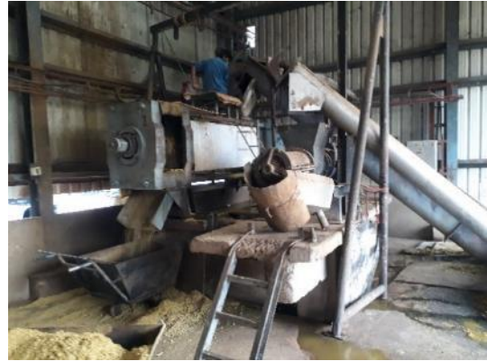
Mixing and blending of cattle dung with undigested food
