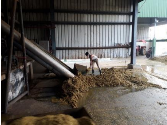
Mixing and blending of cattle dung with undigested food
